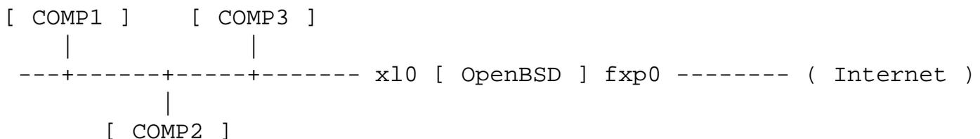
There are a number of computers on the internal network; the diagram shows three but the actual number is irrelevant. These computers are regular workstations used for web surfing, email, chatting, etc., except for COMP3 which is also running a small web server. The internal network is using the 192.168.0.0 / 255.255.255.0 network block.
